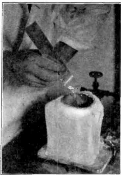
Fig. 4. Melting Platinum in High Frequency Furnace
